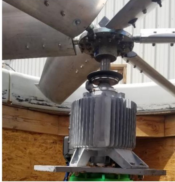
Figure 12: 40HP Direct Drive Transverse Flux Motor on a Test Stand
