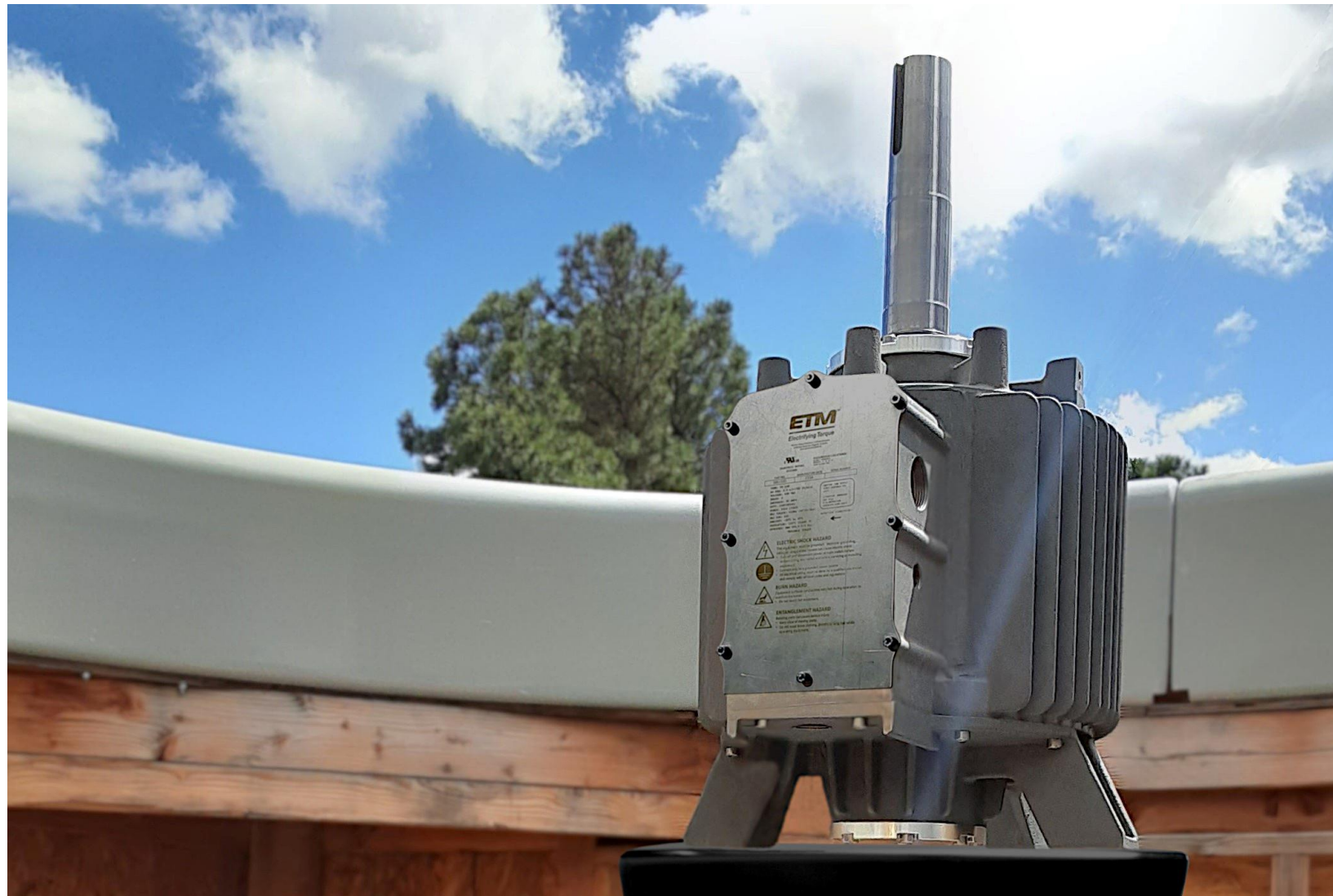
40HP TF Motor 520 Ft-lb (700 Nm) 360 Lbs UL1004, C1D2 Certified
